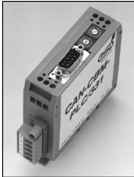
The ISO 11898-compatible CAN interface allows a maximum data-transfer rate of 1 Mbit/s.
